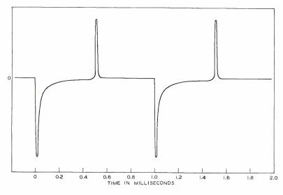
Fig. 5—When the plate current shown in the upper part of Figure 4 is passed through the primary winding of a transformer, the voltage across the secondary winding will be as shown above
