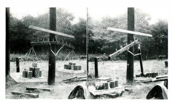
Breaking tests on crossarms at the Chester field laboratory. Test arms were loaded with weights suspended from their ends until they broke
