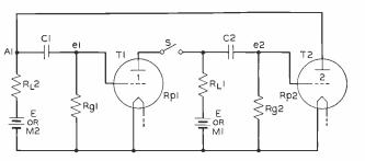
Fig. 3—Simplified schematic of a multivibrator
