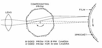
Fig. 2—Schematic diagram of the optical system of the Fastax camera. The prism shown is for the 8-mm model
