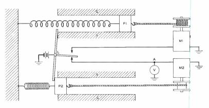
Fig. 2—A multivibrator when represented mechanically becomes more complicated than an oscillator because two moving elements are required, each drawn one way by a spring and the other by a motor, and the surfaces they slide on offer resistance to motion
