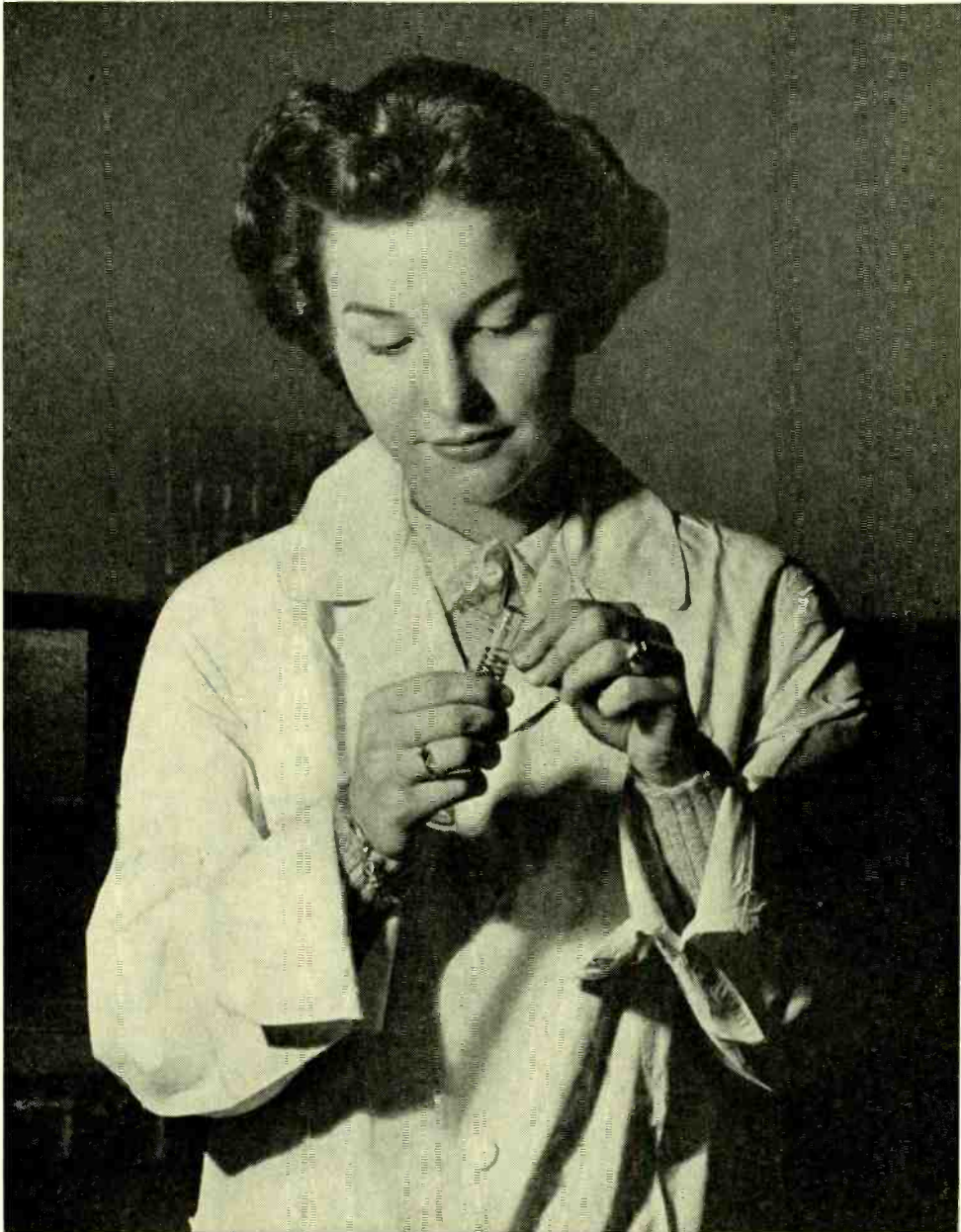
Preparing a protective metal surface for an accelerated corrosion test made over water in a constant-temperature oven
