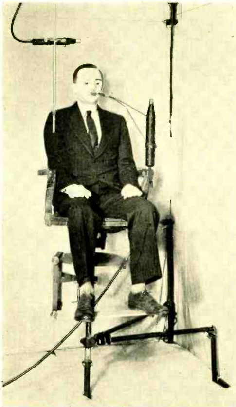
Fig. 1—Arrangement of speaker and microphone for distribution measurements
