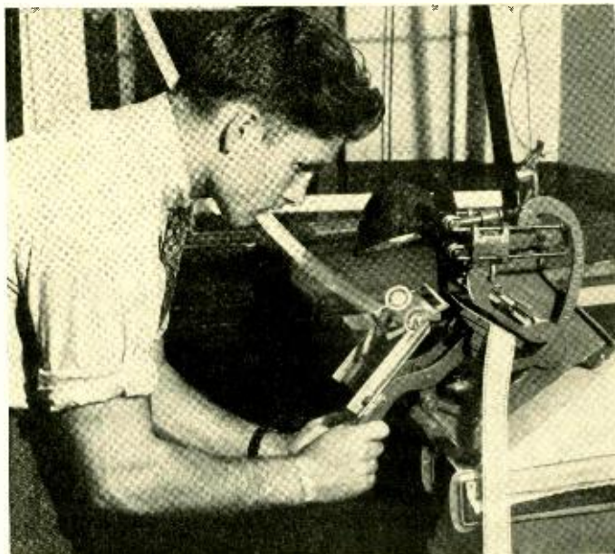
A small hand-operated press is used to print the scale
