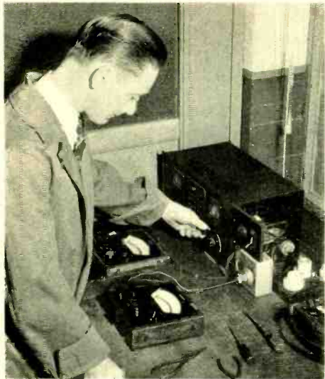
Richard Rafferty checks the accuracy of a meter at the Bureau's test table
