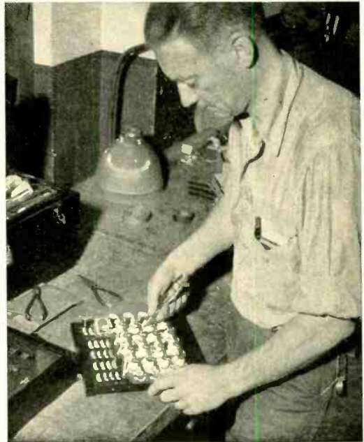
Harry Schucht, an electrician in the Building Shops, modifying an annunciator
