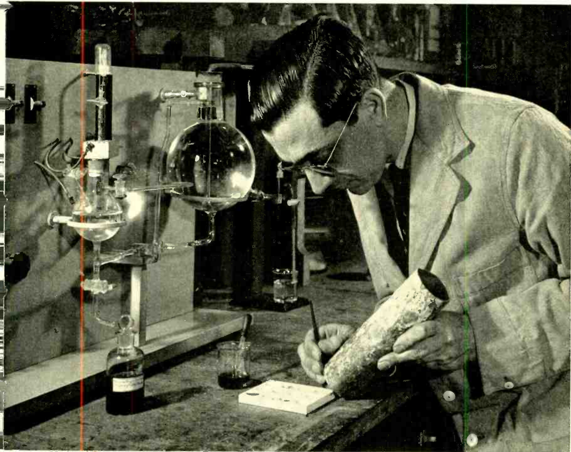
Identifying corrosion product on a cable sheath.
