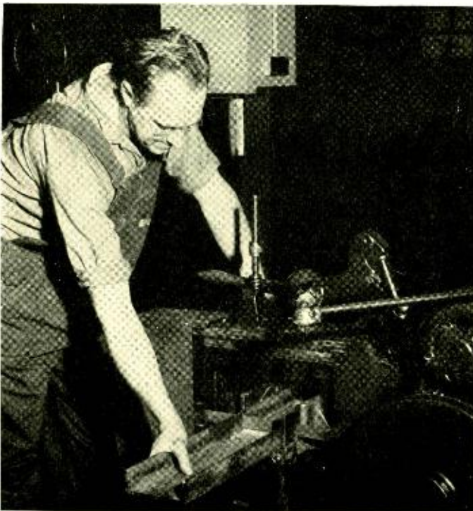
Al Stark of the millwright group cutting a channel iron in the automatic power saw
