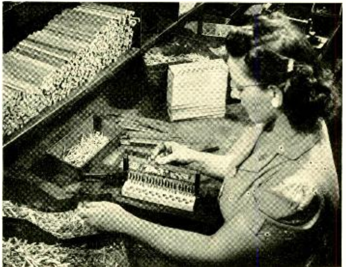
Substituting for critical items on the Nation's list of vital defense materials cuts down on shortages. This Hawthorne girl replaces rubber with wood fibre board in terminal strips for central-office equipment
