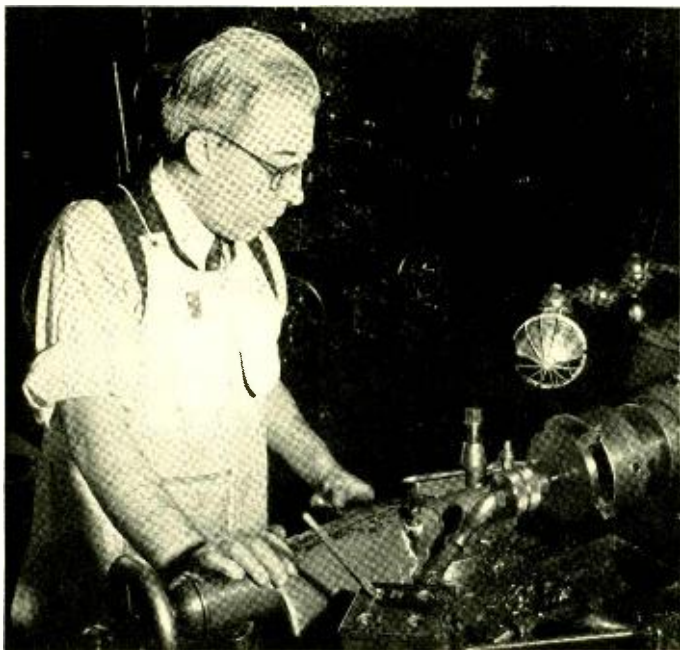
David Anderson machining a permalloy disc on an engine lathe in the Development Shop
