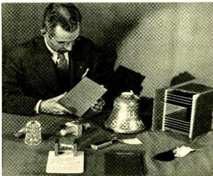
Fig. 1—A group of observational standards including those for finishes, flaws in glass insulators, screw thread fits, color of glass bells, flaws and coverage of the finish on resistors and condensers, and texture of phenol plastic surfaces. C. R. McIver is holding one of the finish standards
