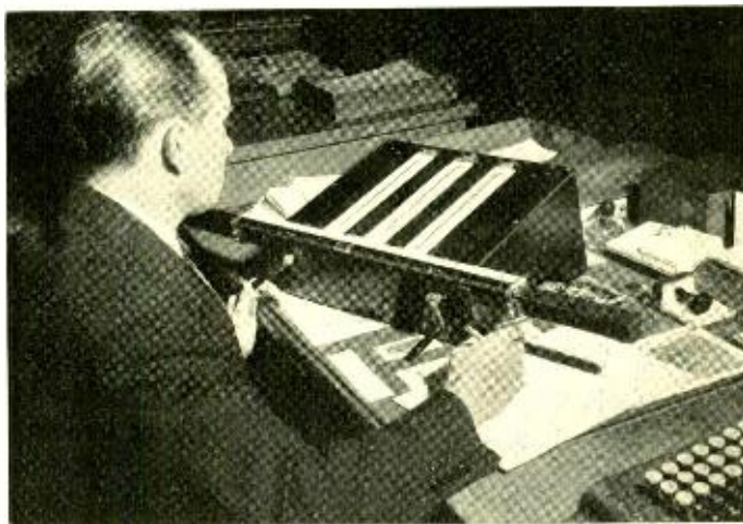
Fig. 6—The point at which new stock should be ordered is computed from tables on rollers in this machine
