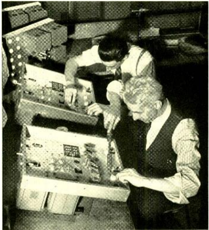
J. A. Boyce and W. F. Besemer assembling and wiring experimental amplifiers in the shop of the transmission development laboratory
