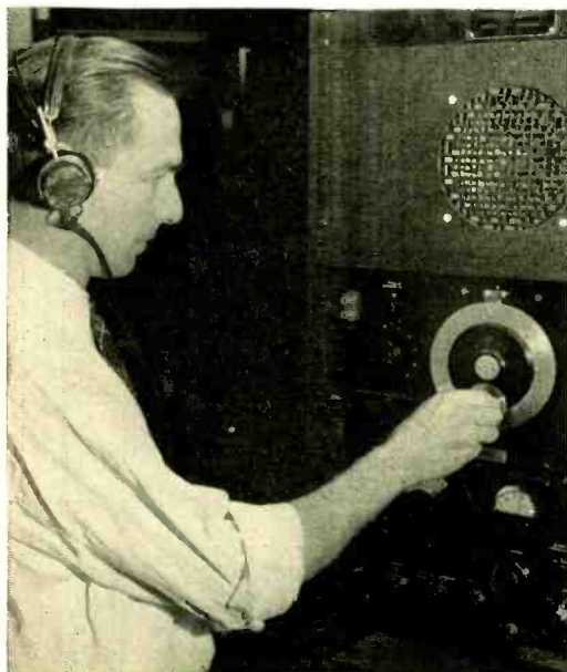
A L. Robinson checking the frequency swing of a frequency-modulation transmitter
