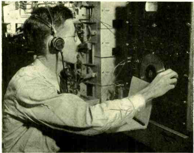
D. B. Penick testing cable-carrier program equipment with a frequency analyzer
