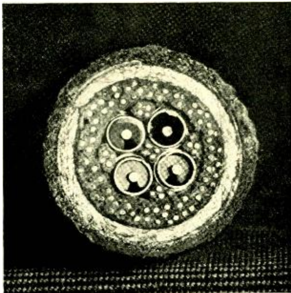
Fig. 5—A cross-section of the Stevens Point-Minneapolis cable reveals the four coaxial structures with two 22-gauge pairs in the central space and one 19-gauge and one 22-gauge pair in each outer interstice between them. Surrounding this assembly is a layer of eighteen 19-gauge quads
