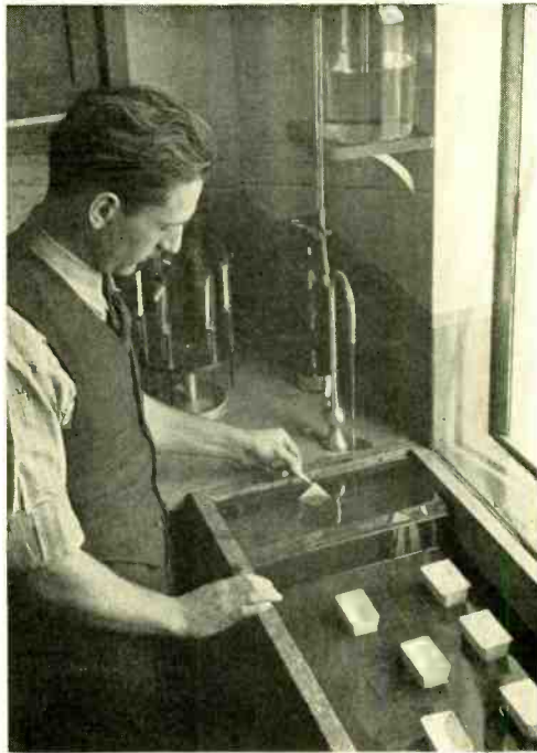
H. V. Wadlow washes out the excess reagent after the print has been developed
