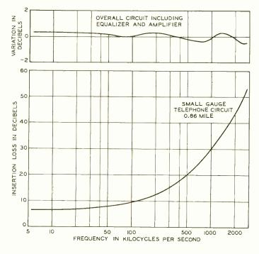
Fig. 2—Overall loss over the television band for a cable circuit plus amplifiers and equalizers
