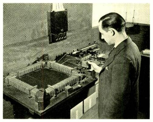
Fig. 3—An Epstein testing set employs primary and secondary windings on a rectangular core made up of specimen strips
