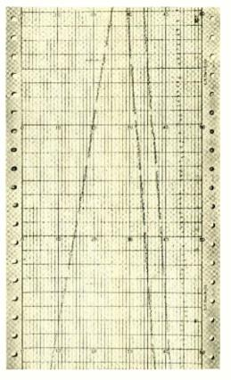
Fig. 2—Chronograph chart. The three records at the left were made by three crystal clocks. The other trace is a record of time signals received hourly by radio
