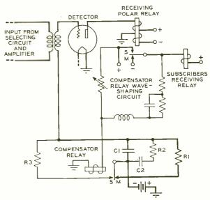
Fig. 3—Complete diagram of level compensator
