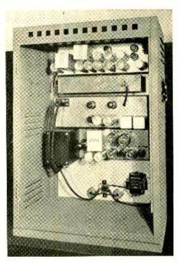
Fig. 5—Rear view of amplifier-equalizer unit with door removed
