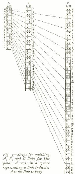
over the hour, and averaging these probabilities together, the result will be the probability that a random call placed at random time during the busy hour will fail to complete. For each time, this requires the matching of each A link with every B and c link with which it may be associated, and noting the paths that because of a busy link are not available.
