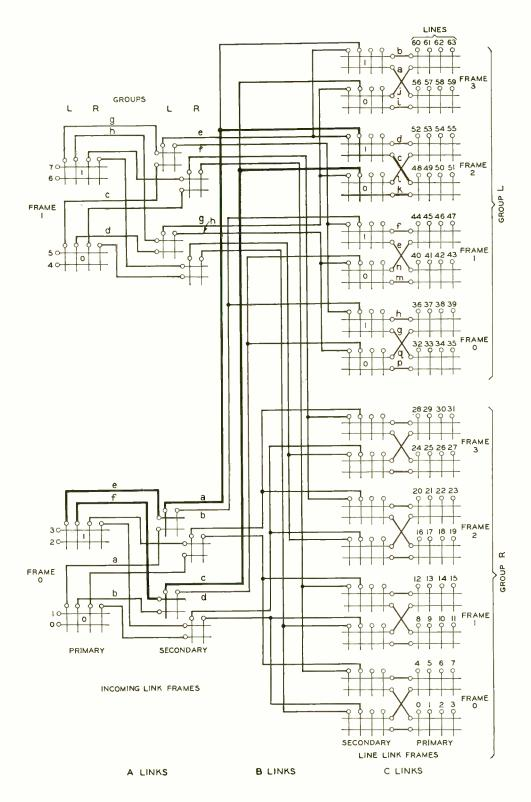
side of the incoming primary switches run to the left side of the incoming secondary switches. The arrangement of the links can be illustrated by considering, for example, a call from trunk 3 to line 48. The two possible A links will be e and f; the B links will be a and c; while the c links will be c and k.
