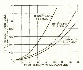
Fig. 4—Core losses in typical materials determined with an Epstein testing set
