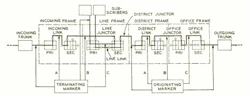
Fig. 1—Block schematic of crossbar system showing ABC trunking scheme October 1939
