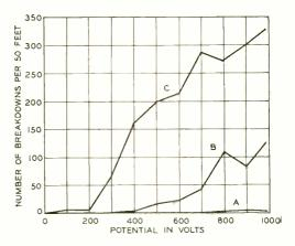
Fig. 4—Wide variations in the quality of the insulation on commercial enameled wire are caused by surface irregularities in the conductor. A, smooth wire; B, intermediate; C, numerous large irregularities
