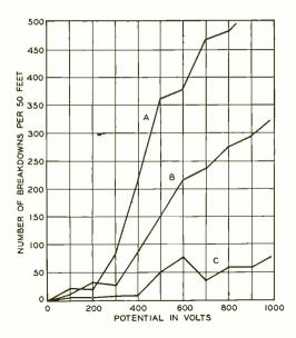
Fig. 3—Thick enamel showed fewer defective places than thin. Thickness—A, .0004 inch; B, .0006 inch; C, .0008 inch
