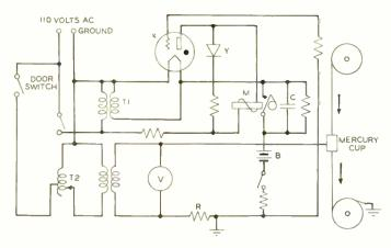
Fig. 1—When the insulation on the wire breaks down at the mercury cup the grid potential of the thyratron tube changes to make it conduct and operate the register M
