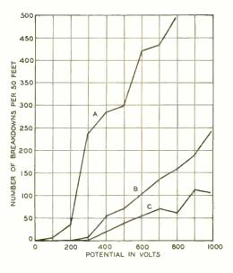
Fig. 2—Enamel wire with smooth conductor showed fewer breakdowns than wire with rough conductor. A, artificially roughened; B, original wire; C, artificially smoothed
