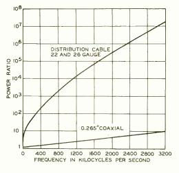
Fig. 1—Losses in one mile of experimental telephone and coaxial-cable circuits over the television frequency range
