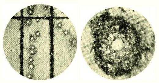
Fig. 3—Photomicrographs of spark records which show the perforations in the chart and the dark rings where the wax was melted by the spark. The divisions on the chart represent hundredths of a second
