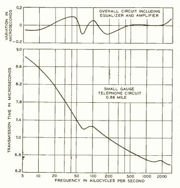
Fig. 3—Time of transmission before and after equalization for the same cable circuit
