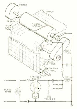
Fig. 1—A metal drum with a spiral raised above its surface rotates above a moving sheet of recording paper which passes over a long knife-edged electrode. Sparks from the knife edge to the spiral perforate the paper at points which depend on the angular position of the rotating drum
