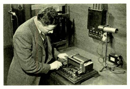
Fig. 5-Clamping a specimen in a Fahy Simplex permeameter
