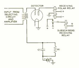
Fig. 2—Schematic of level compensator
