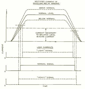
Fig. 1—Telegraph signals of various levels, shown on the upper line, result in received signals of different lengths 46
