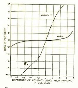
Fig. 4—Improvement in variations in signal bias by the level compensator
