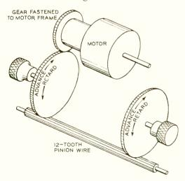
Fig. 5—Gear arrangement for the adjusting drive
