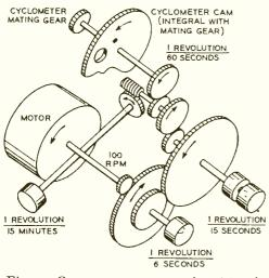
Fig. 3—Gear arrangement used to drive the various commutators
