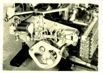
Fig. 1—Holding magnet and selector mechanism of the 15lype teletypewriter
