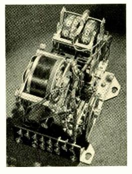
Fig. 1—Time unit with cover removed showing the four timing commutators May 1939
