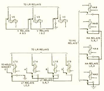
\*RECORD, April, 1939, p. 234. Fig. 5—Typical chaining circuits of the line-link controller May 1939 271
