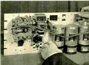
These two models, representing different stages in engineering the 2B Regulator, were built in the Shop. "Breadboard" models were built, but have not survived. As soon as such a model has served its purpose, it generally is disassembled and the apparatus used in a new circuit. The 2B Regulator, shown at the right, occupies but nine inches of space on a standard relay rack. An entire C5 carrier terminal, including the regulator, is mounted on one bay, as shown below.
