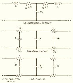
Fig. 2—Equivalent networks for longitudinal circuit, above; phantom circuit, center; and side circuit, below
