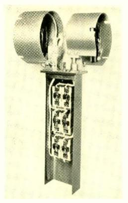
Fig. 4—Partially assembled loading coil case potting six 81A filters
