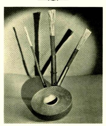
In improved cable for inside wiring which has better moisture-resisting characteristics than similar cable now in use is shown here. The improvement results from the addition of a thermoplastic jacket between the core of the cable and the braid. This jacket makes unnecessary a cord under the braid to aid in stripping; and it permits the cable to be made with a smooth surface and more pleasing appearance.
