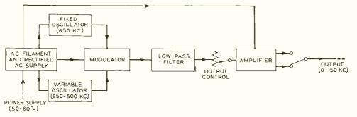
Fig. 1—Block schematic for the 17B oscillator
