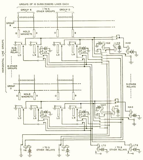
Fig. 3—Simplified schematic indicating the relays involved in line identification May 1939
