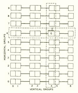
Fig. 2—Any of the seventy possible groups of ten subscriber lines can be identified by specifying the horizontal and vertical groups
