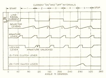
Fig. 3—Timing of the cams of the selector-cam assembly. The relationship between the line signal and the operation of the several cams can be varied by repositioning the rangefinder arm of the mechanism
