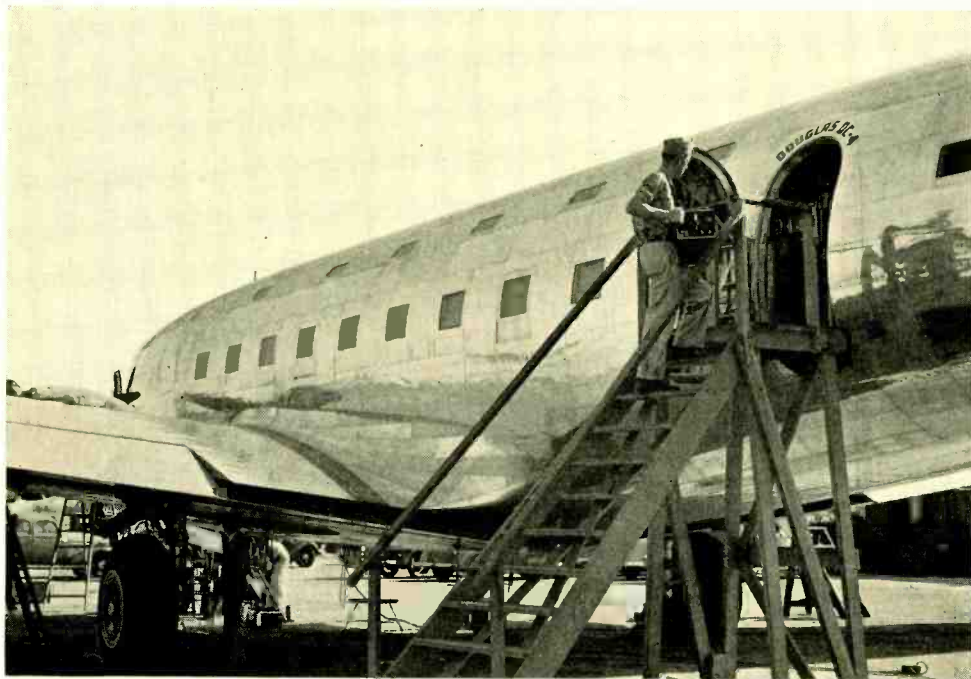
This Western Electric radio receiver, which is being installed on the giant Douglas DC-4 transport plane, is part of the most elaborate radio system yet developed for air service. It includes separate receivers for communication, beacon, weather and marker services, and a 250-watt transmitter. As the ship passes through the five radio zones of the transcontinental route, the transmitter and communication receiver to which it is geared are shifted progressively through five pairs of "day" and "night" frequencies, by means of a crank with an indicating dial on the transmitter panel
