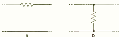
Fig. 3—The expanded metal form of acoustic resistance corresponds to a series electrical resistance as at "a," and the "washer" form corresponds to a shunt or absorbing resistance as at "b"
