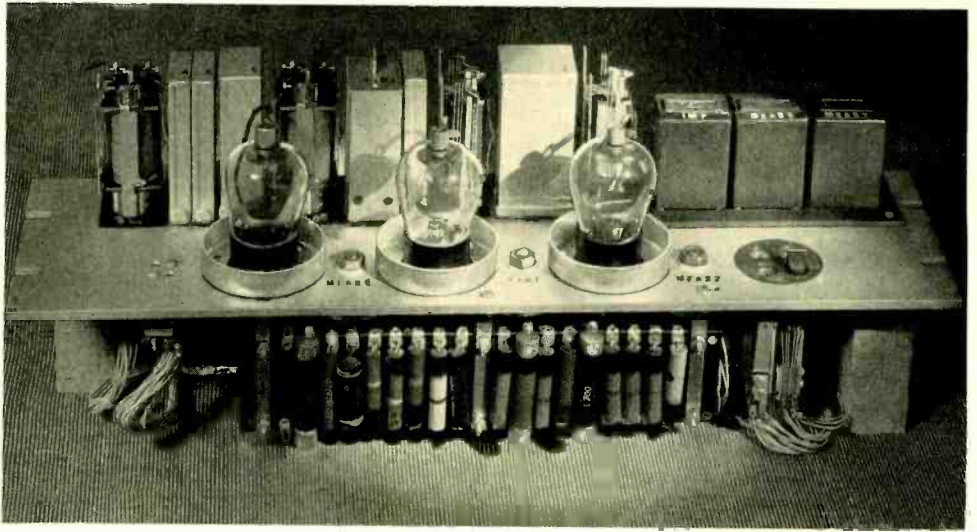
Fig. 2—Rear view of a two-stage voltage recorder which is equipped with message registers and a time-delay circuit
