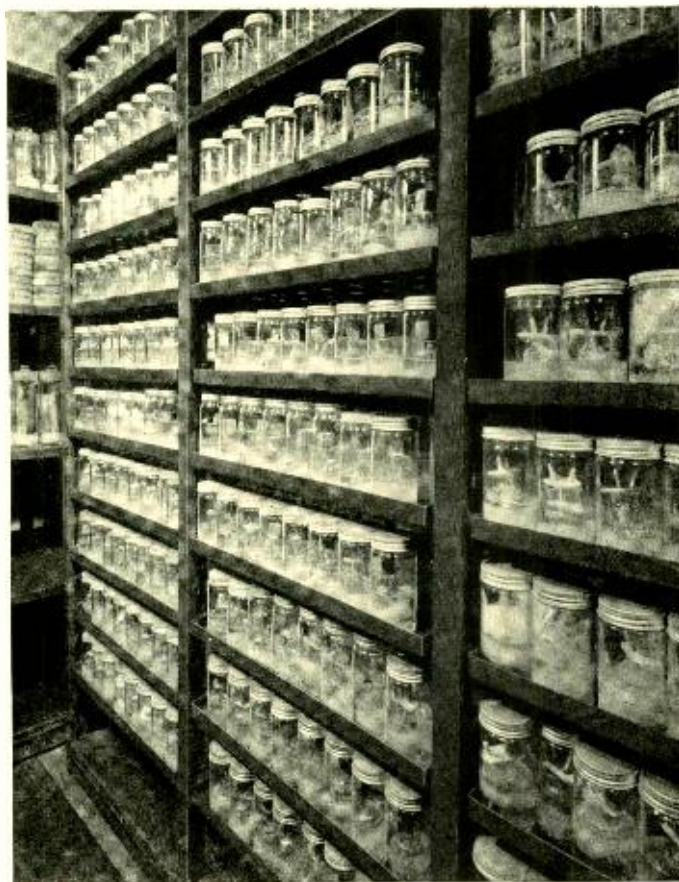
Fig. 4—Incubation room where the bottles are stored during the twenty-four-week test period at a constant temperature of twenty-six degrees Centigrade
