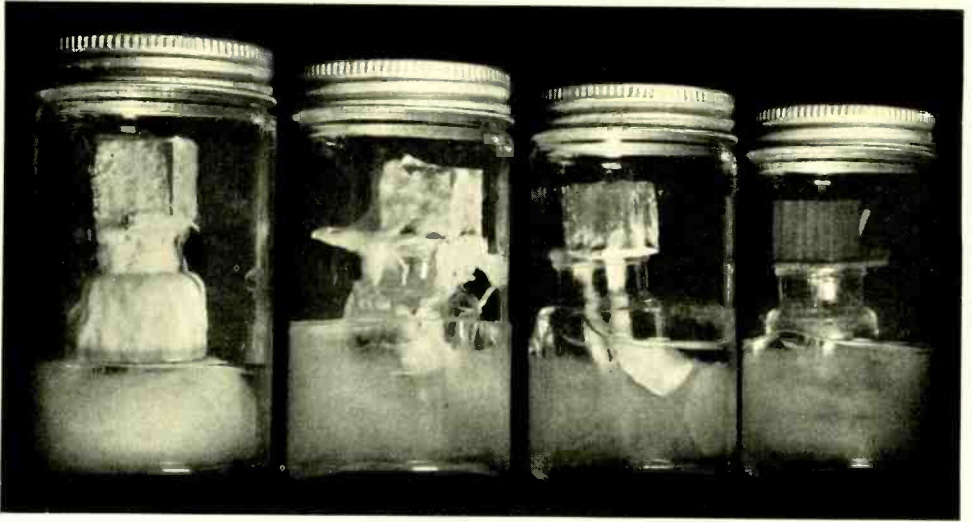
Fig. 5—Test of a preservative with the wood-block method showing the effect of increasing concentration on the growth of the test fungus Lenzites trabea . Growth ratings of these typical test blocks from left to right are 4-4, 4-3, 3-2, 0-0
