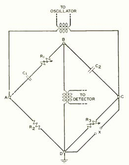
Fig. 1—Simplified schematic diagram for the product-arm bridge
