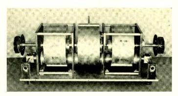
Fig. 1—The electrical path through the high-frequency attenuator, shown here with its dust cover removed, is a straight line through the lower part of the three drums
