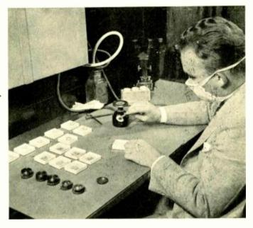
Fig. 1—.4 special suction tool permits the diaphragm to be handled during assembly without touch by the hand
