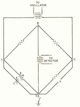
Fig. 2—Simplified schematic of the precision-comparison type bridge
