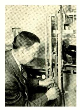
Fig. 2—W. A. Bunzel adjusting the vaporpressure thermostat and humidostat
