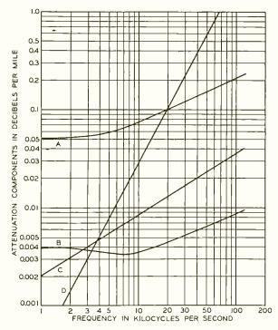
Fig. 1—Attenuation losses on open-wire lines. A, series loss; B, change in series loss for 20 degrees Centigrade change in temperature; C, shunt loss with CS insulator in moderate rain; D, shunt loss with one centimeter of ice on wires
