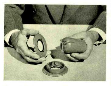
Fig. 2—The baffle consists of two disks with a leather washer between them, which holds the baffle to the microphone
