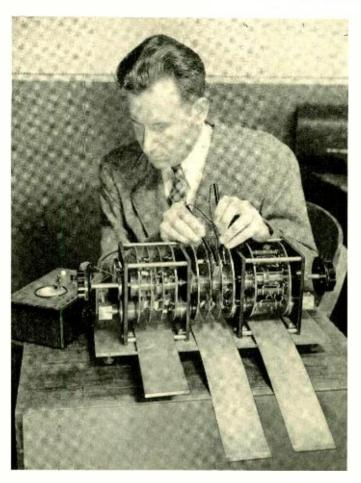
Fig. 2—For the low-loss units on the decade drum, the three resistances forming each of the T-networks are wound on a single spool; for the higher-loss units two or three T-sections are used which are wound on spools with shields between them
