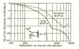
Fig. 6—Decrease in response at 150 degrees relative to that at zero degree, both with and without the baffle
