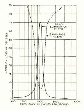
Fig. 3—Characteristics of the band-pass and band-elimination filters
