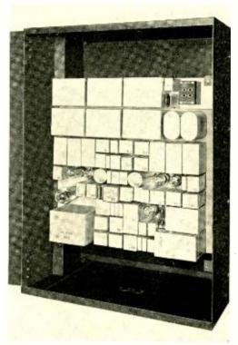
Fig. 2—The type-H terminal may be installed either on a relay rack bay or in a metal cabinet as shown above
