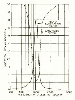
Fig. 3—Characteristics of the band-pass and band-elimination filters
