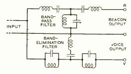
Fig. 4—Schematic of the 724A filter unit
