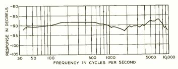
Fig. 4—Response characteristic of 633A microphone for sound at 90-degree incidence
