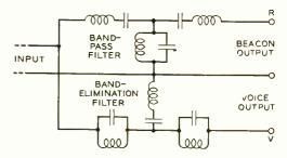
Fig. 4—Schematic of the 724A filter unit
