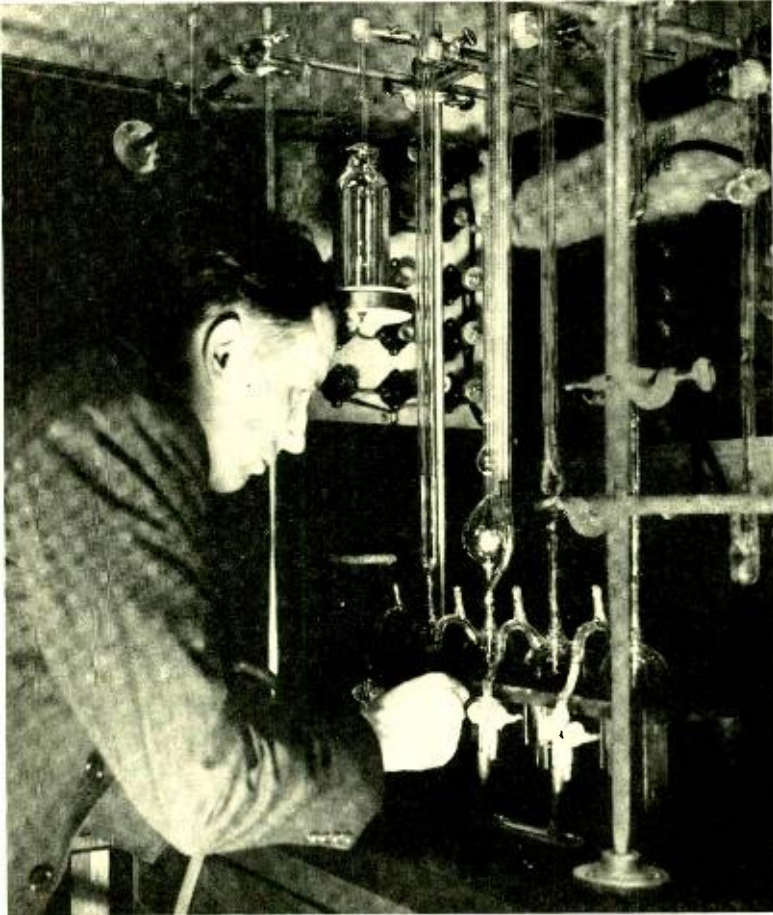
Studying the gases generated by the thermal and electrolytic decomposition of paper
