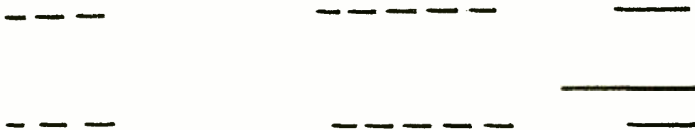
Fig. 2—Record made for a call to line 35; above, not busy; below, busy
