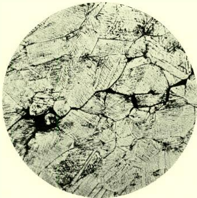
Photomicrograph of a section of a telephone gong that has suffered corrosion cracking. The failure is intercrystalline, and the surrounding structure is plastically strained
