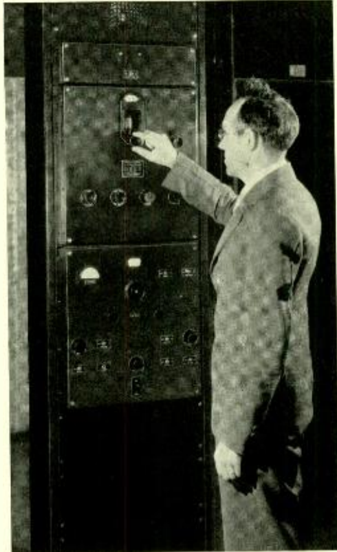
Fig. 1—Setting the radio-frequency tuning dial at the frequency to be measured prior to making a frequency measurement
