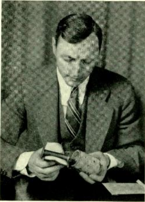
Fig. 1—A. P. Fahn demonstrates the heater and heating element of the carbon monoxide detector for manholes
