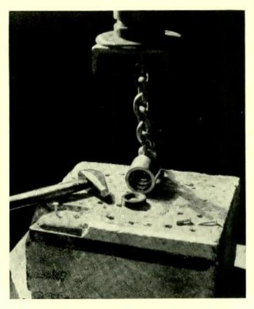
Laboratory test for masonry anchors
