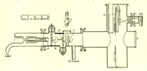
Fig. 4—Longitudinal cross-section of the electron diffraction camera March 1936
