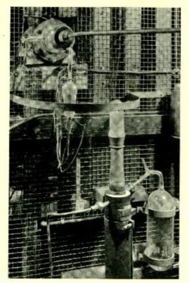
Fig. 2—The filament end of the camera. The filament is maintained at a potential of 50 or 60 kilovolts negative to ground. The transformer, rectifier, and filter which supply the high negative potential to the filament are shown in the headpiece
