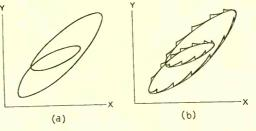
Fig. 3—The oscilloscope pattern (a) is changed to that shown at (b) when the relaxation oscillator is applied, thus indicating in this case that the oscilloscope spot is actually rotating in a clockwise direction
