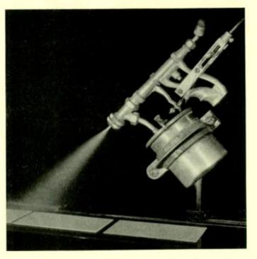
Fig. 2-Several panels can be sprayed simultaneously
