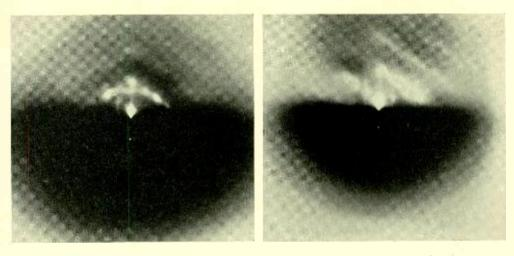
Fig. 3—Diffraction patterns from oriented layers of stearic acid molecules
