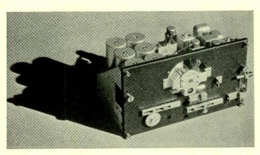
Western Electric 20-type radio receiver developed by the Laboratories to provide a light, compact set of extreme selectivity for use in small aircraft. The receiver is designed for either remote (shown above) or local control and is provided with four frequency bands covering a range from 200 kilocycles to 10,000 kilocycles
