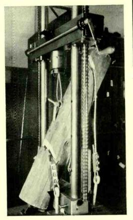
Fig. 1—Storm guy straps used on telephone poles are tested under service load conditions by mounting them on a section of a pole held at an angle in an Amsler testing machine
