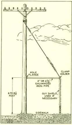
Fig. 4—A horizontal iron pipe is used to prevent the guy strand from interfering with the right-of-way
