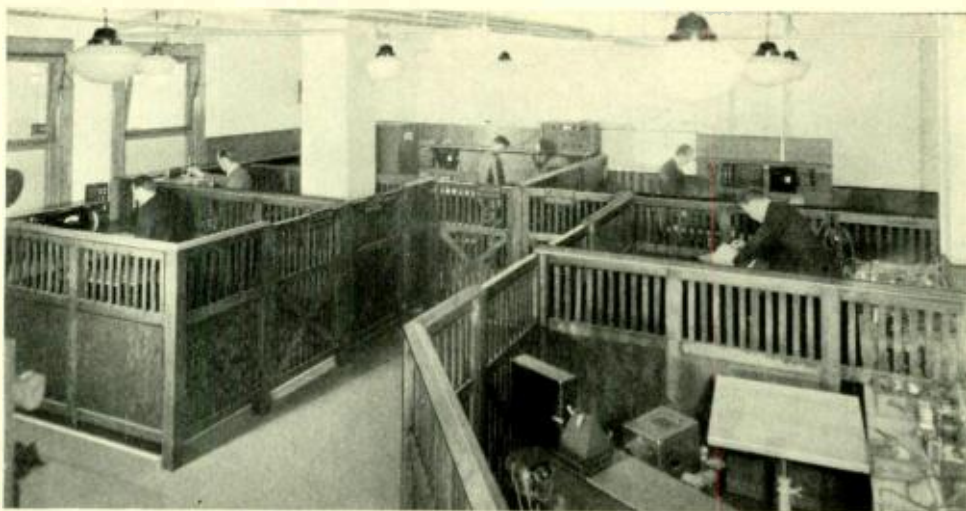
Fig. 3—The compartments are similar in having a bench, writing stand, and outlet boxes for power supply, but vary in size and in their special equipment
