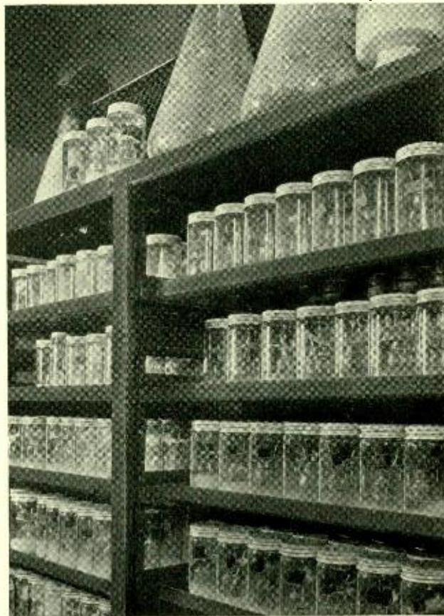
Testing wood preservatives by rotting treated blocks, using a special technique developed in the Summit Laboratories
