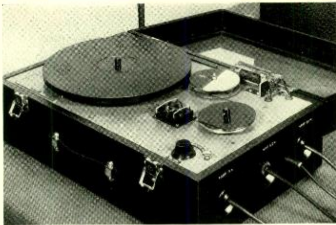
Fig. 2—The recording and reproducing halves of the switching cam are colored respectively black and white, so that a speaker can readily observe the position of the cam and know how much longer he may talk
