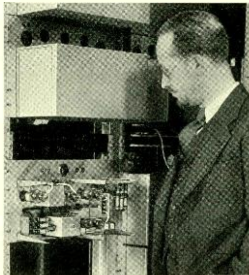
Fig. 7—C. L. Weis with a group modulator for use in a million-cycle terminal
