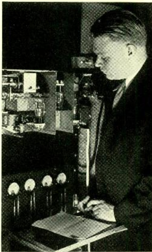
Fig. 5—K. C. Black with a high-frequency repeater developed for coaxial circuits
