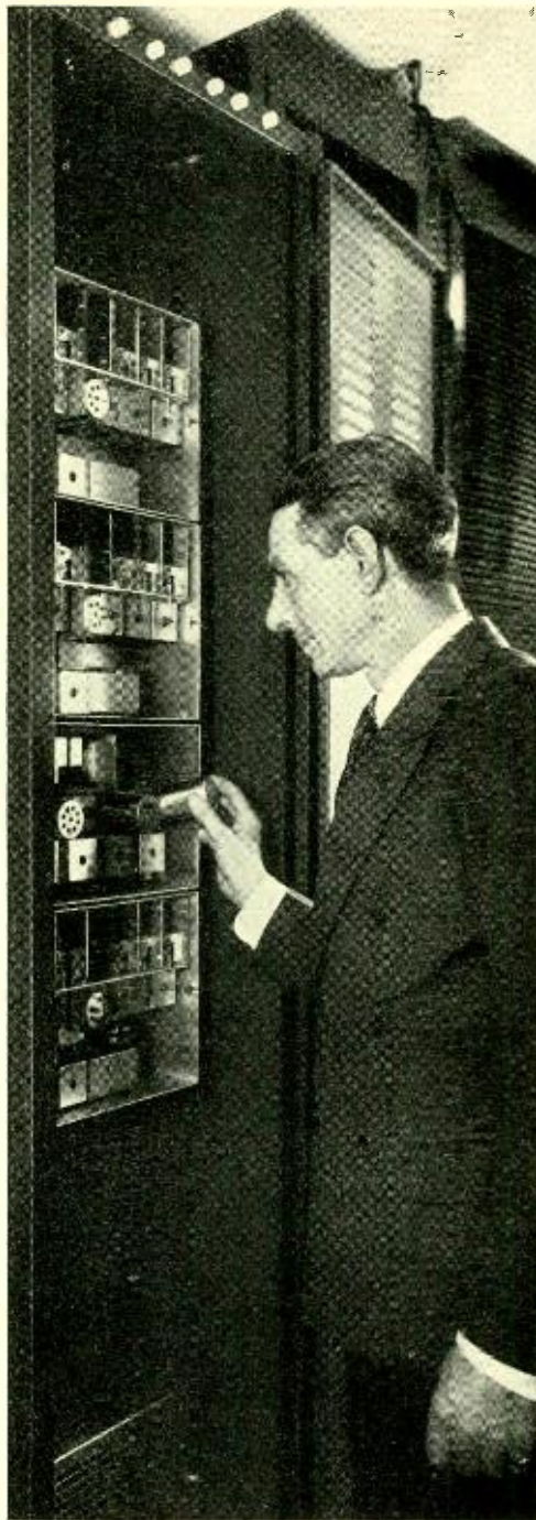
Fig. 5—In the intermediate-frequency amplifier, shown undergoing inspection by J. Stevens, Radio Technician of the Waldorf, the power of the signal is increased a hundred thousand million fold
