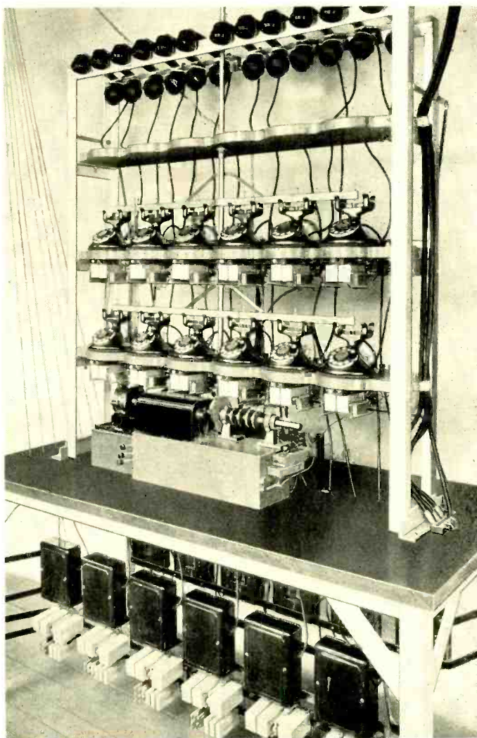
Fig. 3—The study of contact trouble in subscribers' handset mountings was facilitated by a machine which operates the switchhook contacts under proper circuit conditions, and stops itself when the resistance of the contacts exceeds a predetermined value
