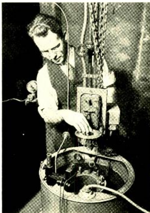
Fig. 1—G. G. Winspear placing samples of moisture-proofing membranes in a bomb where they will undergo accelerated oxidation, to test their life properties
