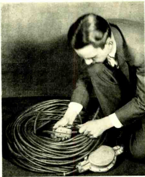
Fig. 1—Cable terminals are of moulded rubber with brass bushings and screws
