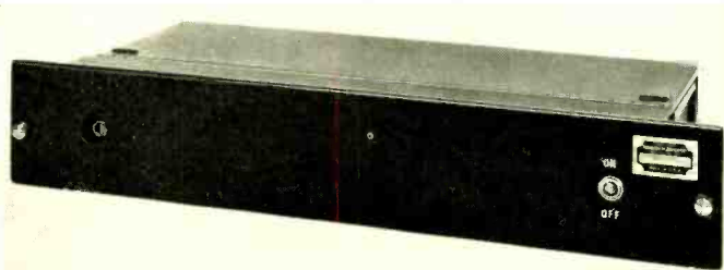
Fig. 1—Nothing appears on the front of the panel of the 80A amplifier but a power switch and a testing jack
