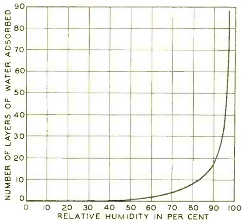
Fig. 1—McHaffie and Lenher have shown that a clean washed surface of glass adsorbs a film of moisture whose thickness in terms of molecules varies with the humidity as shown above
