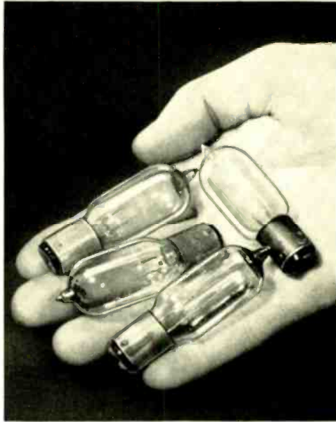
Fig. 6—The new ballast lamp, employing a two-contact Edison base, is of unusually small size
