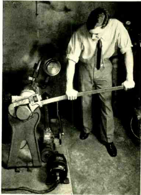
Fig. 1—Closing the autoclave in which the raw materials for artificial anthracite were pretreated at low temperatures
