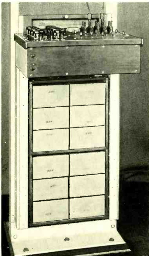
Fig. 1—Front view, with front panel and foot rail removed, showing the associated battery consisting of twelve 22½-volt units, behind which is located the galvanometer
