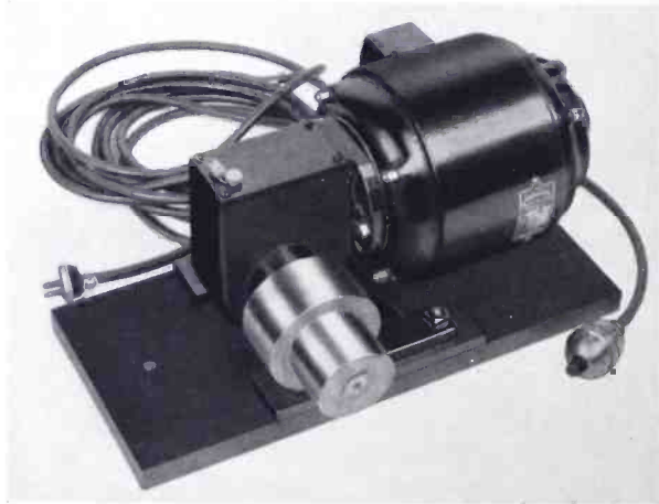
Fig. 2—A small driving motor is provided mounted on a wooden base which is braced against the frame of the main machine while in operation
