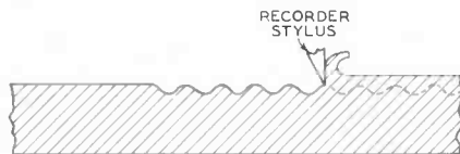
Fig. 4—A schematic indication, not to scale, of the difference between lateral and vertical records
