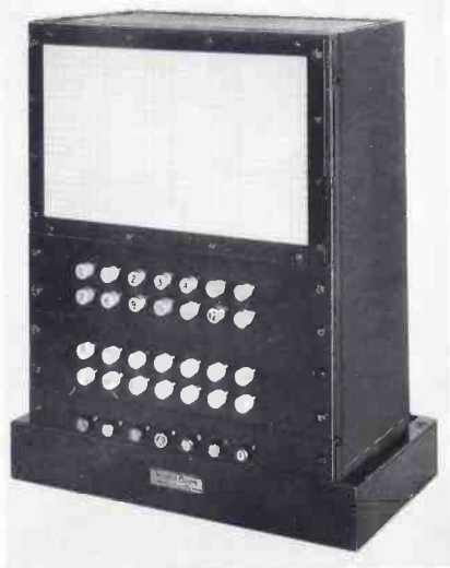
Fig. 4—On the upper part of the calling equipment, in front of the space occupied by the synchronous motor and the rotating brush, is a designation card for listing the various codes
