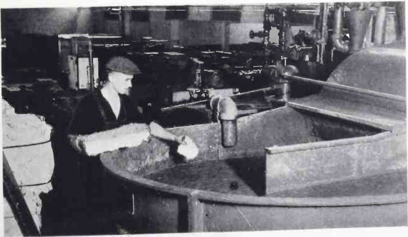
Fig. 1—Pulp is thrown into the beater, kneaded with water, and then dumped into the storage tanks beneath
