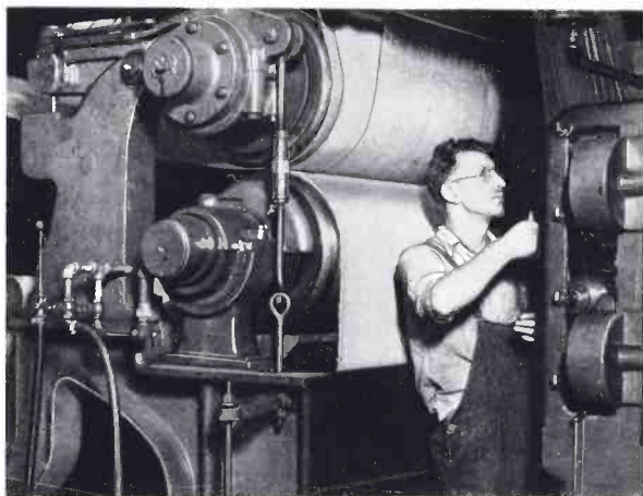
Fig. 2—The wires embedded in ribbons of wet pulp leave the press rolls (center) and enter the polishing machine (right)
