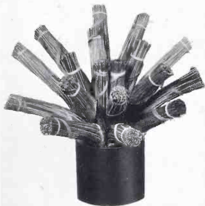
Fig. 4—This 1800-pair No. 26-gauge cable illustrates the application of unit stranding to pulp-insulated cable
