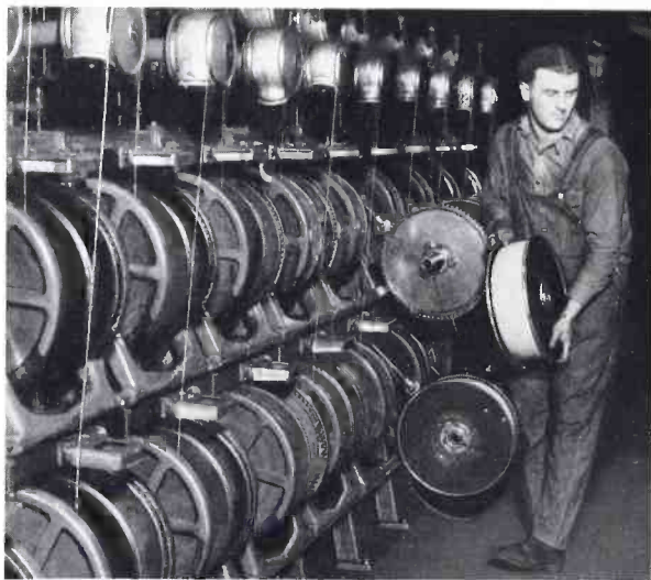
Fig. 3—The finished insulated wire is spooled beneath the drier
