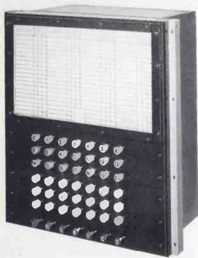
Fig. 3—The 63-type selector key has 21 keys in each group instead of fourteen
