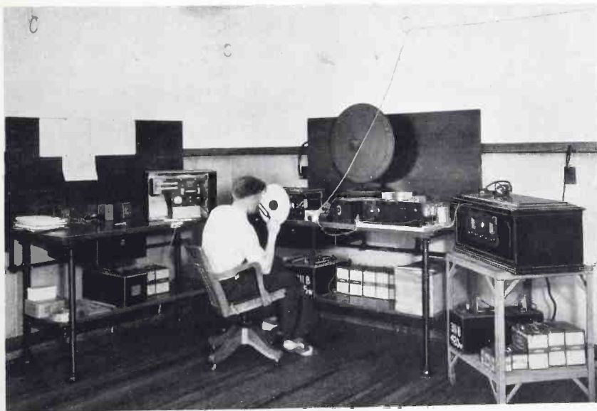
Fig. 3—J. P. Dolbear at the Mendham Laboratories measuring the frequency of a distant airplane radio station
