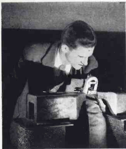
Fig. 3—Magnetizing a loudspeaker magnet between poles of electromagnet
