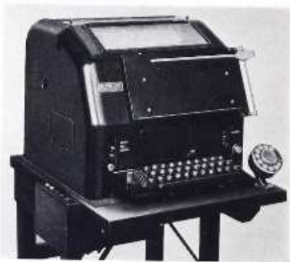
Fig. 1—In the current installations of the selective calling system, a teletypewriter of the No. 15 type is used. Control box and dial are mounted adjacent to it
