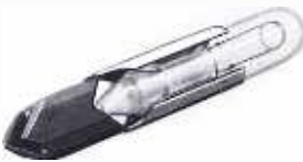
Fig. 1—All switchboard lamps of the present time, although differing widely in voltage, current, and illumination characteristics, have similar outside dimensions
