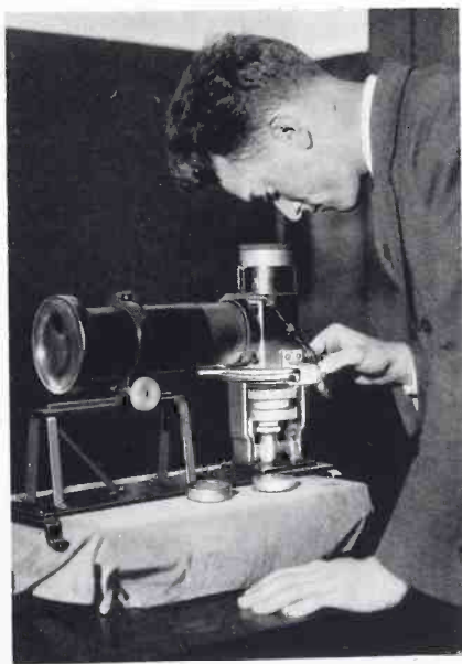
Fig. 4—Flatness of the back plate of a condenser transmitter being measured on a large field interferometer
