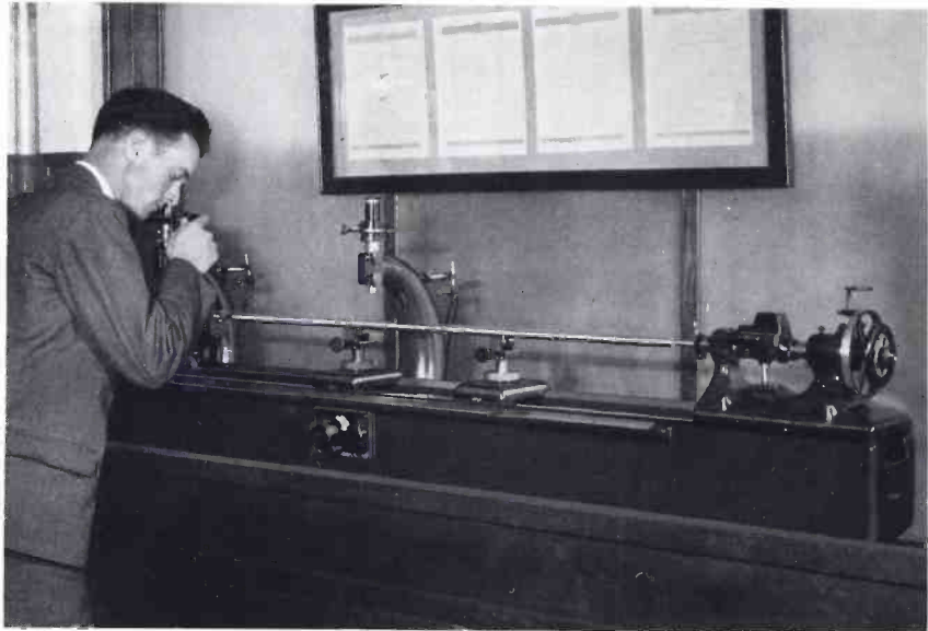
Fig. 1—R. O. Sloan making a precise length determination of a steel rod
