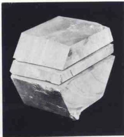
Fig. 1—Slab for thickness vibration cut from large crystal
