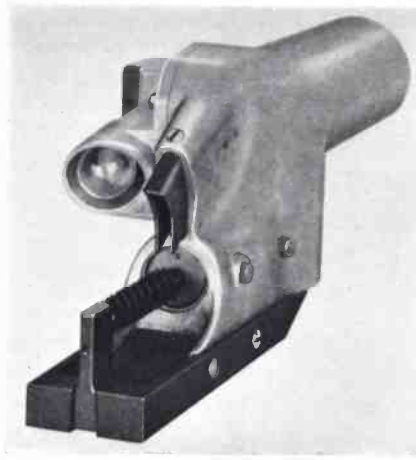
Fig. 1—The new cleaning tool incorporates a power-driven brush, a vacuum cleaner connection, and an electric lamp in a cast aluminum housing
