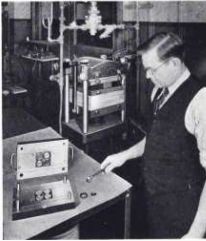
Fig. 4—E. L. Dias of the Chemical Laboratory removing one of the rubber membranes of the new transmitter from the mold
