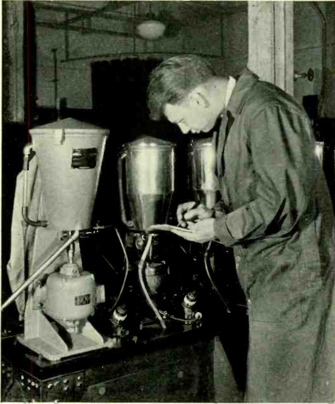
Testing wear-resisting qualities of finishes in the Laboratories
