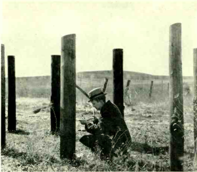
Fig. 5—G. Q. Lumsden securing a sample from a creosoted pine post
