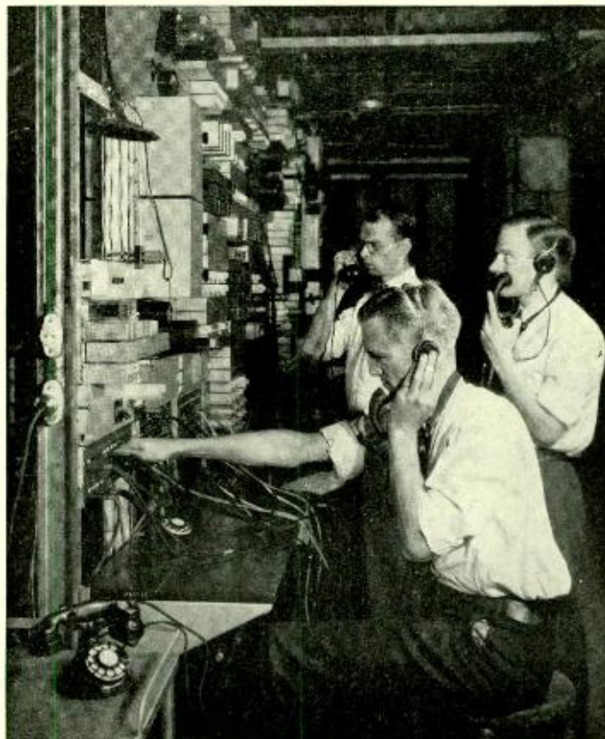
Experimental terminal apparatus in the Systems laboratory, through which a call was dialled from Chicago to the Canal central office in New York during Mr. Grace's recent Chicago lecture
