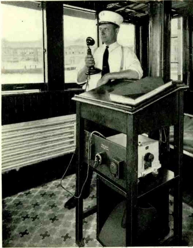
Captain George J. Baum of the New York Fire Department speaking through the radio-telephone equipment in the pilot house of the John Purroy Mitchell. Note the loudspeaker under the shelf supporting the receiver
