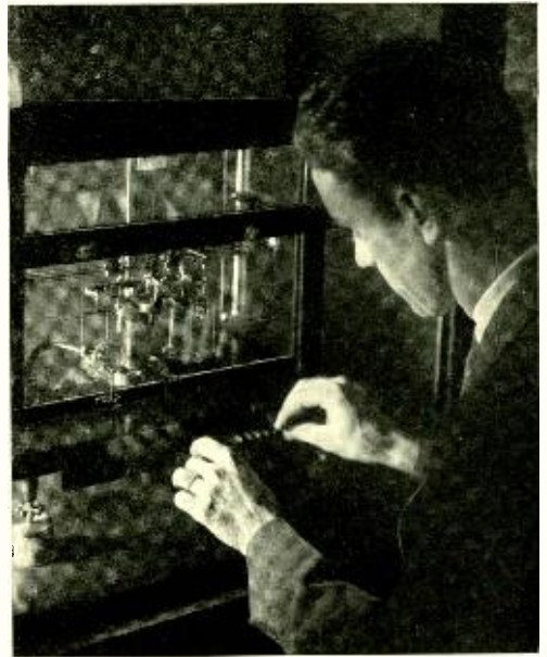
A balance accurate to one five-hundred thousandth of a gram! It is used in the work under H. T. Reeve and is being operated by R. S. Sclater
