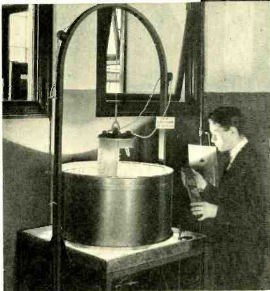
Below, H. A. Johnson studying a sample that has been subjected to the action of the accelerated weathering machine
