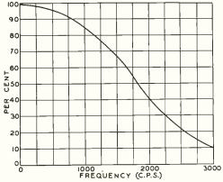
Fig. 2—Syllable articulation when energy below given frequency is suppressed
