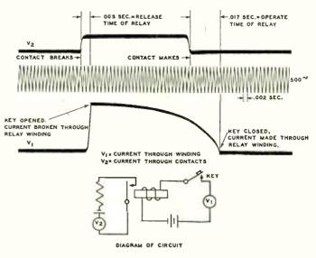
Fig. 1 — Oscillogram showing "operate" and "release" times of a relay in a typical circuit
