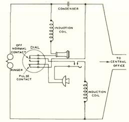
Wiring diagram for subscriber's set showing how dialing opens the circuit
