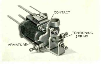
Fig. 3—Having, like the L type, very fast "operate" and "release" times, the stepping or 207 relay is used for but one purpose in the Bell System
