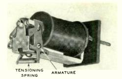
Fig. 4 — The 208 type or counting relay; one of the high-speed relays of the Bell System
