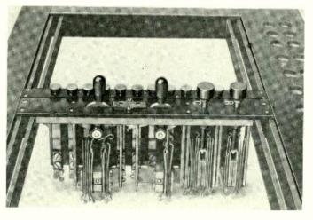
An A-2 type key mounted in a keyshelf, with the posts between the mounting strips at front and back of the shelf
