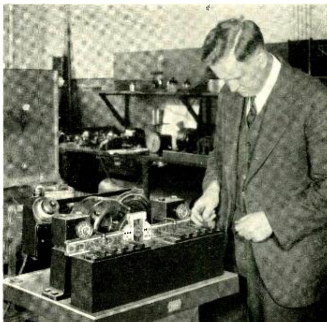
A machine built in the Laboratories for fatigue tests of sheet spring material, and W. S. Hayford, its designer
