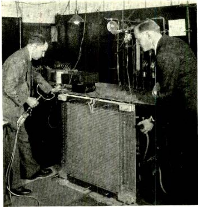
Pumping one of the big neon-tube grids: C. T. Wood manipulates the hand-fire while H. W. Weinhart measures the pressure in the tubes
