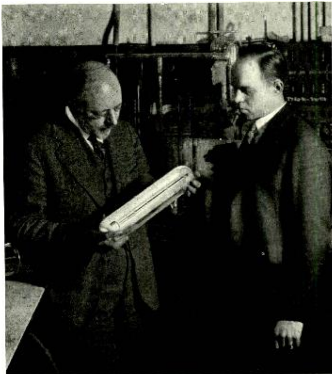
One of the giant photoelectric cells, which serve as eyes in television, is being examined by Herbert E. Ives from whose researches it arose. At the right is G. R. Stilwell who assisted in its production
