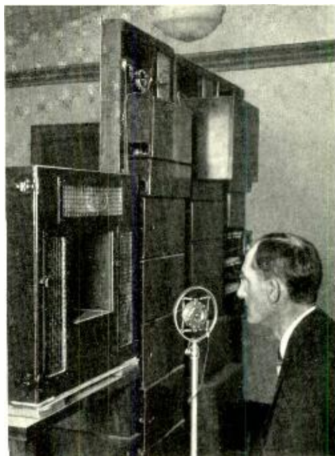
A close-up of the transmitting apparatus for television at Washington. E. F. Kingsbury as he talks to the microphone is viewed by three photoelectric eyes located behind the three screens of the box immediately in front of him
