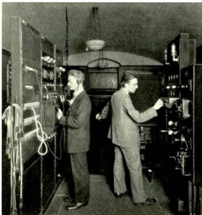
The nerve center of the photoelectric eyes of the television equipment installed at Washington. G. R. Keith and J. G. Knapp of the Laboratories manipulate the controls at the amplifiers which transmit the scene to New York
