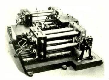
Machine for vibrating short lengths of cable. Cracking of any sheath admits air to a partial vacuum in the samples; a mercury manometer then closes its contact and indicates that a failure has occurred
