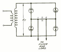
Fig. 4-A circuit which uses four elements
