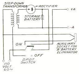
Fig. 6—Typical "trickle-charger"
