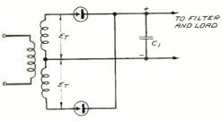
Fig. 3—A simple form of full-wave rectifier
