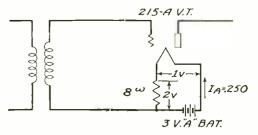
Fig. 9—11ow a grid bias can be supplied by potential drop in a filament circuit
