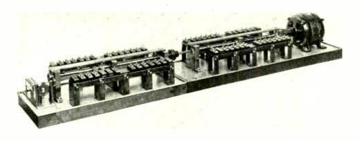
Fatigue-tester with a capacity of fifty-six specimens of sheath material
