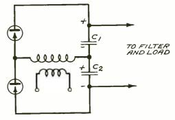
Fig. 5—A two-element rectifier for higher voltages
