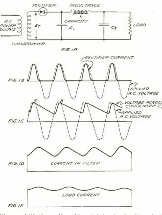
Fig. 1—A "half wave" rectifier; (a) its circuit; (b, c, d, e) wave-forms of current and voltage
