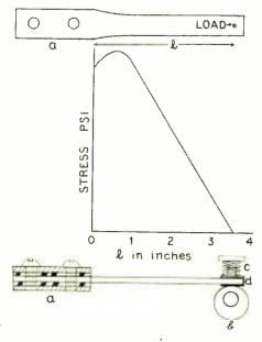
A sample; distribution of stress in it, and how the stress is applied
