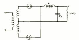
Fig. 2—Another form of filter from which the condenser  $G_1$  has been removed
