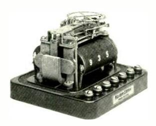
The 60-A selector: as the armature vibrates, it advances the wheel from which stop-pins are seen projecting downward
