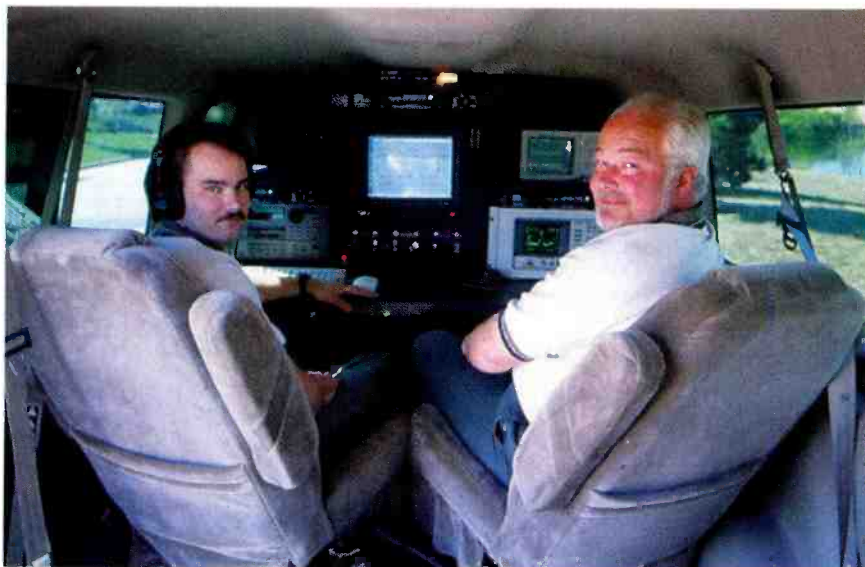
USADR engineers Derrick Clerici (l) and Keith Ege use this test van to monitor the strength and clarity of IBOC signals from commercial-radio partner stations located in Baltimore and Washington.
