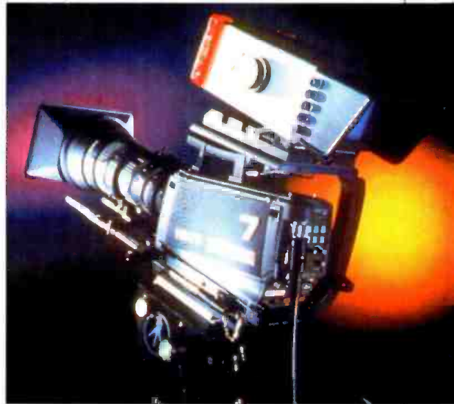
The Philips BTS PTC-9000 750-line progressive scan camera, developed in conjunction with Polaroid, takes pictures at 60 frames per second and supports the 720 P transmission standard.
