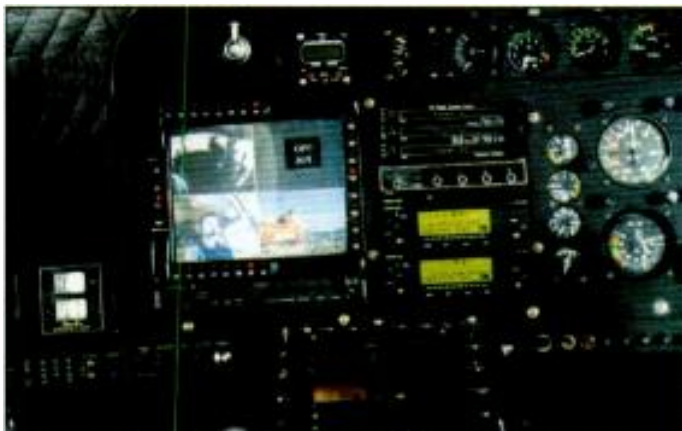
Geneva's quad-screen video system. Two screens allow the pilot/reporter to preview video sources; one shows the station's broadcast, or 'air,' and the fourth shows the signal being transmitted.
