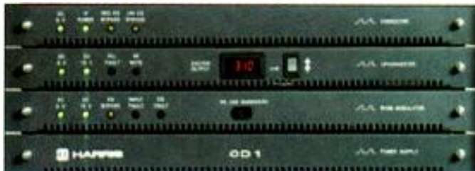
Harris Corp.'s ATV digital exciter will be used in both tube and solid-state models.
