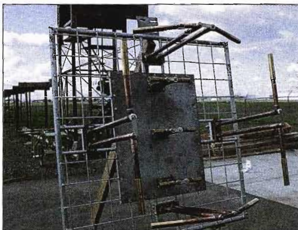
The business end of Jampro's dual-mode NTSC/HDTV antenna that can also send VHF and FM signals at the same time.
