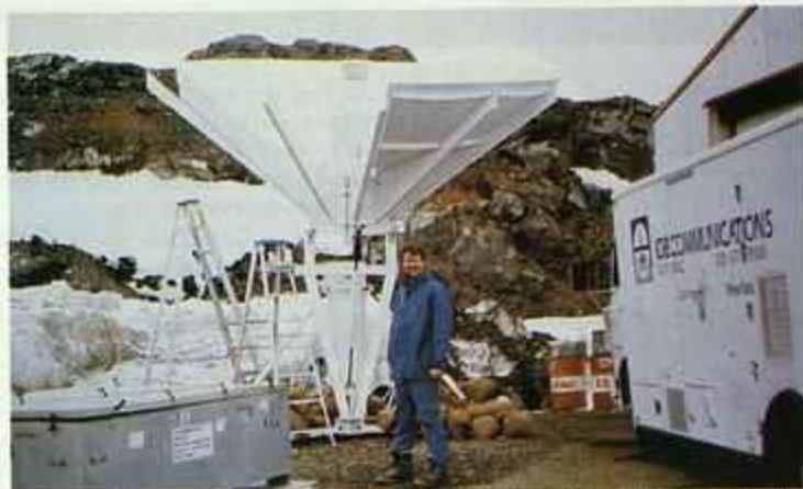
IDB Broadcast used a C-130 transport plane to deploy what might be described as the world's largest flyaway satellite earth station—35,000 pounds of truck and 4.5-meter C-band antenna—to King George Island off the coast of Antarctica for Nippon Television's New Year's Eve special, featuring Japanese mountain climber Junko Tabei. IDB technicians Steve Johnston (pictured) and Scott Grose manned a facility that required Inmarsat phones and external generators.
