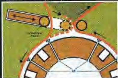
• Tape guide retracts for threading ease • Air drum eliminates head contact in shuttle/standby modes
