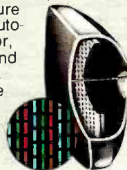
JVC In-line black stripe picture tube.
