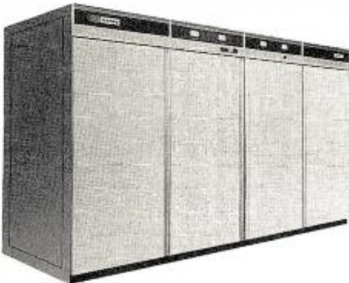
MW-50, 50 kW AM transmitter: We threw away the modulation transformer and reactor.
