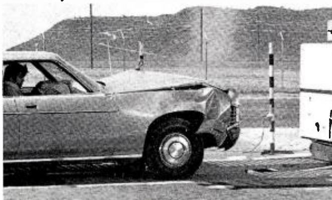
Air bag deflates within 1/2 second. Passenger uninjured.
